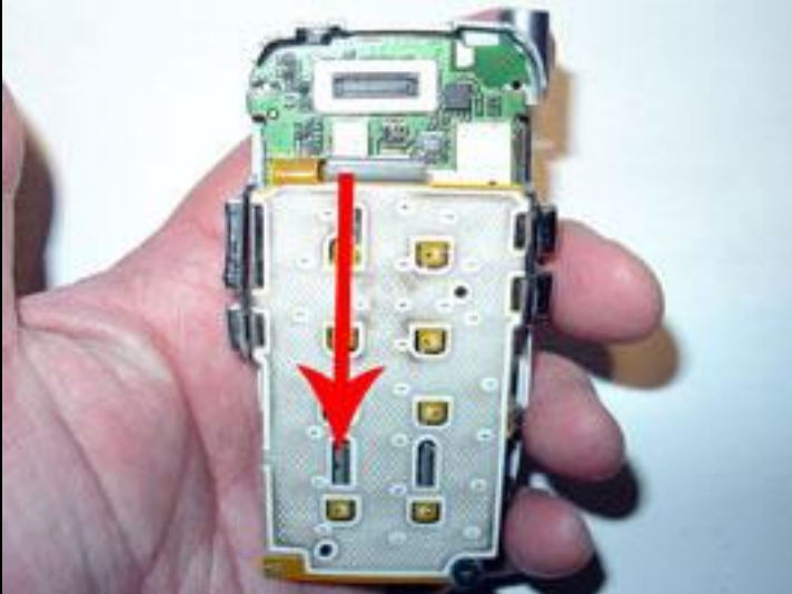
3) Gently slide the keyboard down, so you can clearly see the flex cable connector
