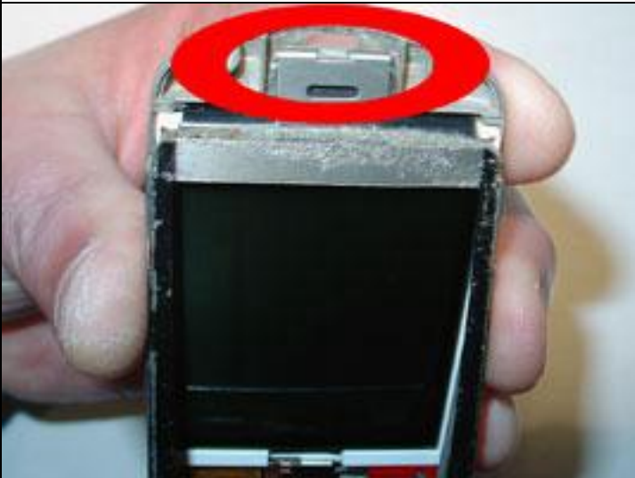
11) Match up the hole on top of the earpiece with the notch on top of the housing, then slide the entire LCD unit back into place
