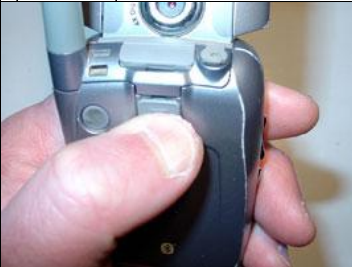
5) Properly secure the battery cover .. check
