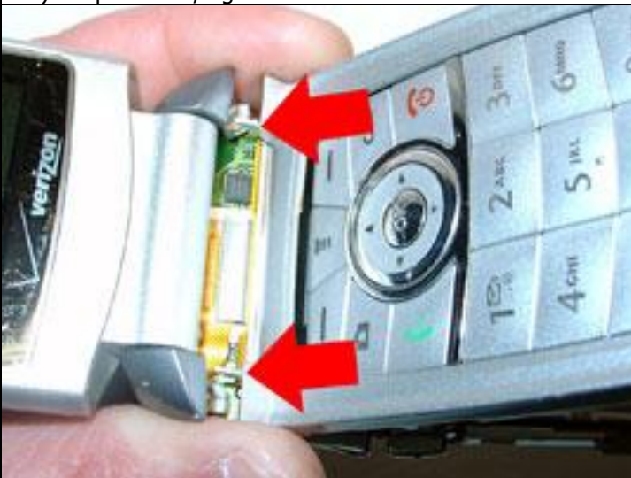
17) There are two little notches on the keypad housing that hold it securely under the hinge, you do NOT want to break these!
