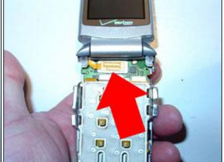
4) Attach the flex cable back into the connector. Either hold around the hinges tightly, or keep the upper housing level, so that the flex cable doesn't break
